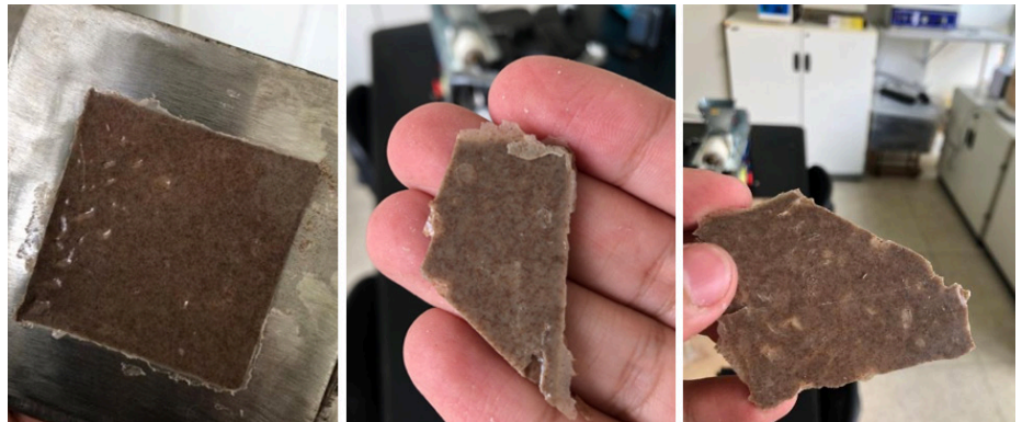
Figure 09. Sample of 90% PLA + 10% PEG/Fiber 75.
