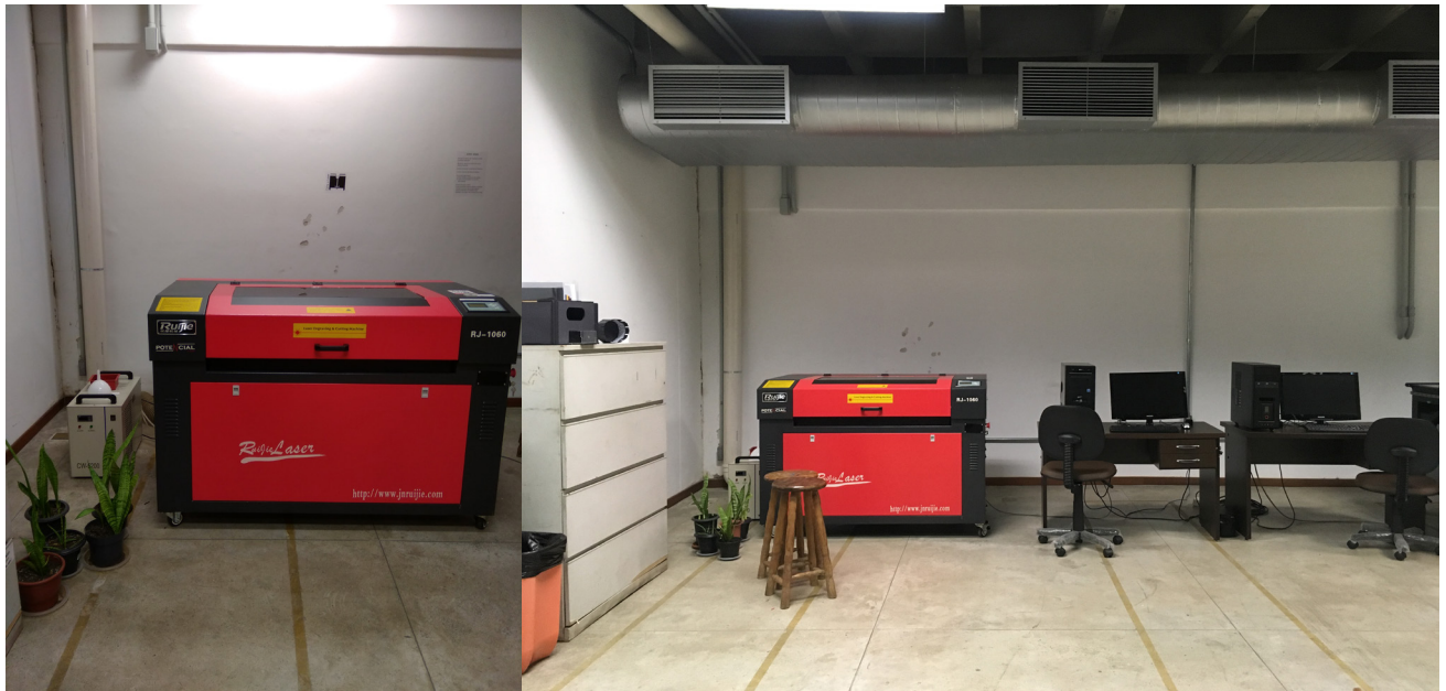
Figures 2a (detail), 2b (general view) Ruijie laser cutter, model RJ-1060. Modeling and Digital Manufacturing Laboratory (ModelaFab), Espaço das Artes (EdA), University of São Paulo (USP), São Paulo. Source ModelaFab team.
