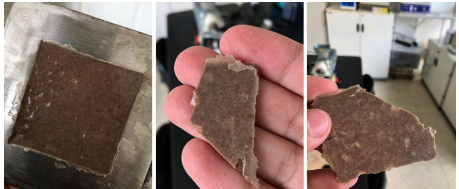
Figure 09. Sample of 90% PLA + 10% PEG/Fiber 75.
