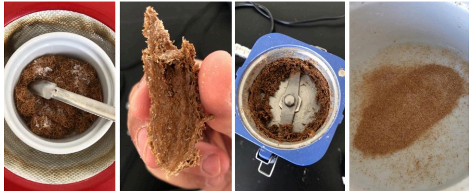
Figure 06. Process of mixing Polyethylene glycol with acai fibers.
